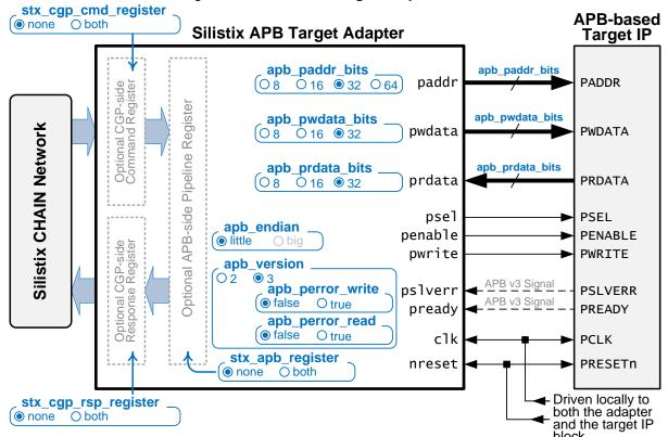
Figure 4: Silistix APB Target Adapter and Attributes
