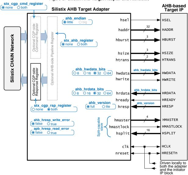
Figure 6: Silistix AHB Target Adapter and Attributes
