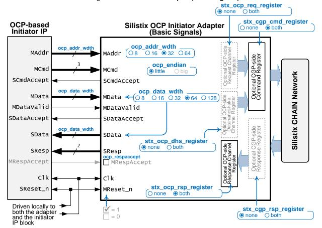
Figure 9: OCP Initiator Adapter (Basic Signals)
