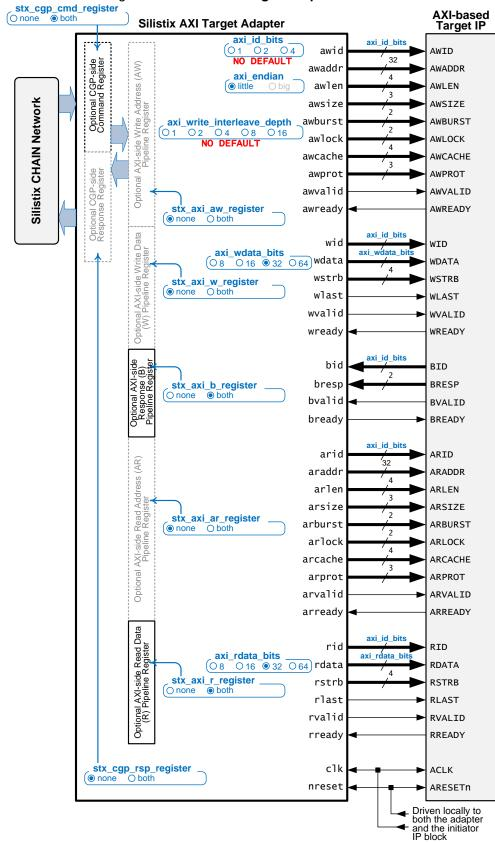
Figure 8: Silistix AXI Target Adapter and Attributes
