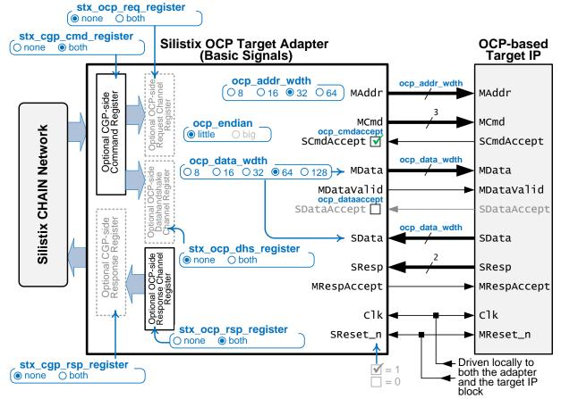
Figure 10: OCP Target Adapter (Basic Signals)
